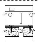
Direct Screw from Above Ceiling Grid 15/16" [24 mm] T-Grid
